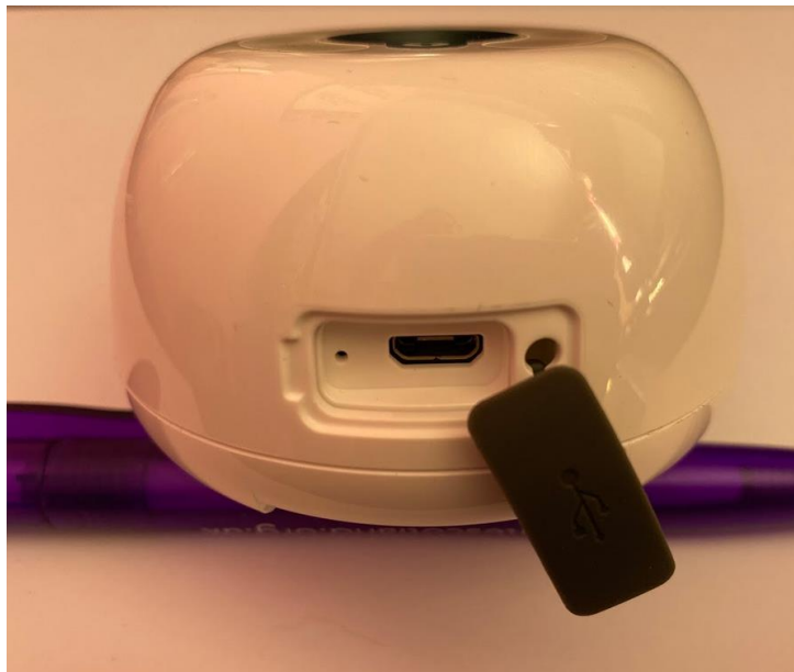
Figure 6 - Image of the Micro-USB peripheral and the reset button
