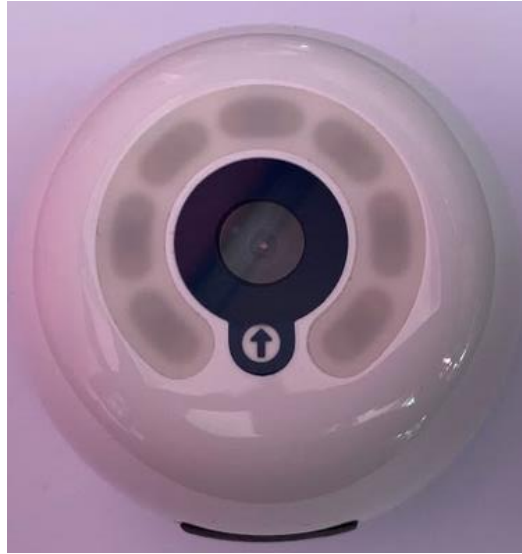
Figure 7 - Top of the FridgeCam where the camera and LED ring are situated
