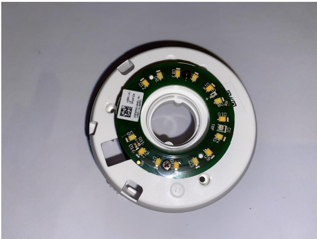
Figure 17 - LED's used for flash
